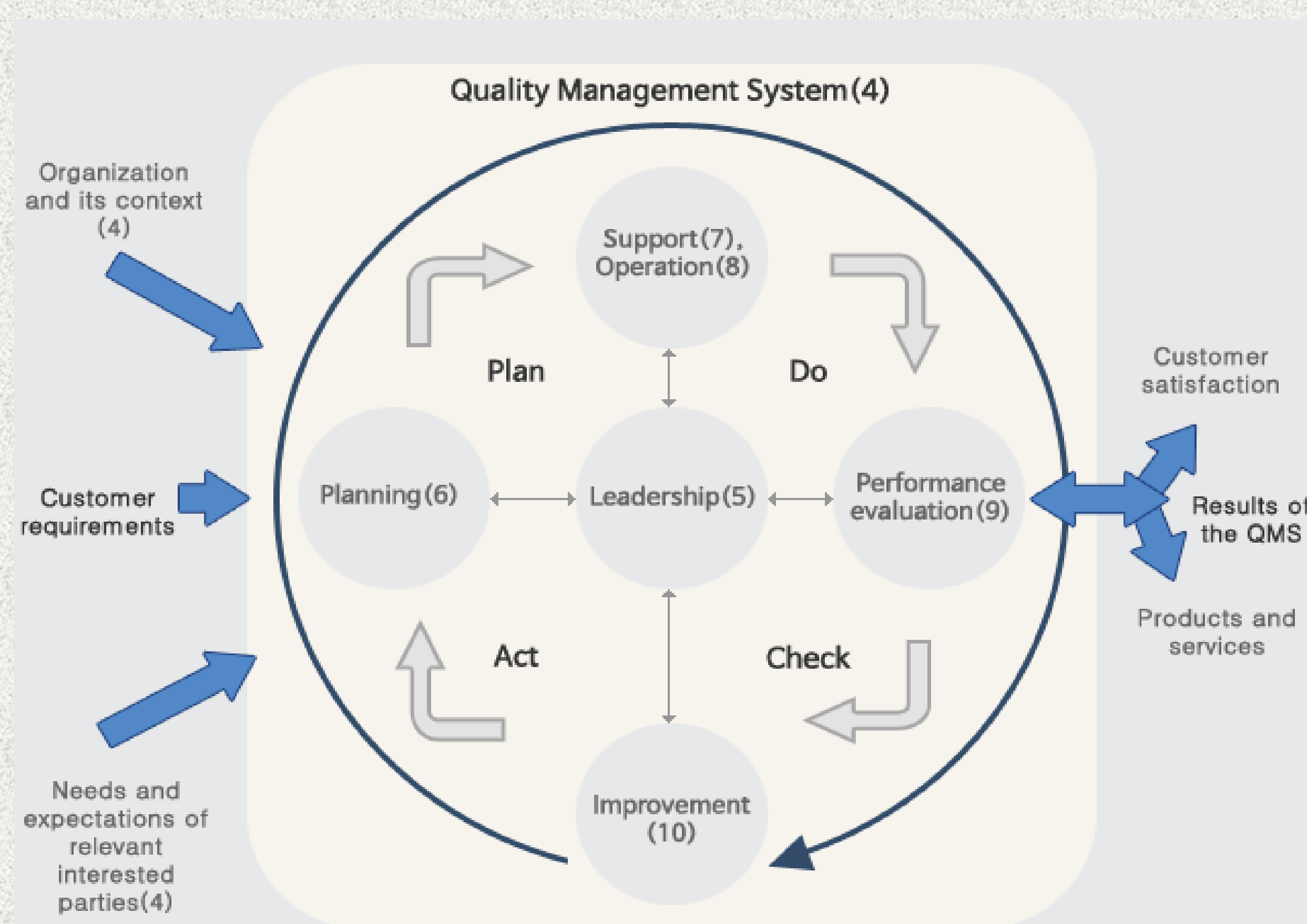
Structure of ISO 9001 in PDCA cycle – Number in brackets refer to the clauses in this International Standard
